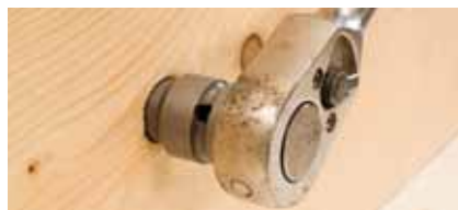
6. Release insertion sleeve with ratchet.
