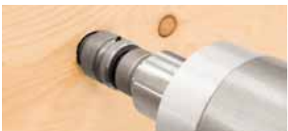
5. Countersink WB directly with insertion sleeve.
